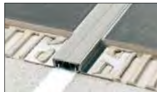
Schlüter®-DILEX-KSBT is a structural movement profile with edge protection, consisting of side anchoring legs of aluminium or stainless steel connected to a 20 mm or 30 mm wide movement zone of soft synthetic rubber. (Product data sheet 4.19)
