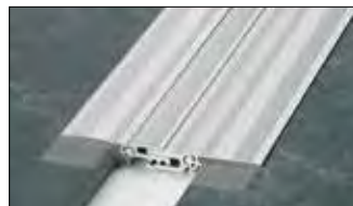
Schlüter®-DILEX-BTS is a structural movement and control joint profile made of aluminium for retrofitting in finished coverings. The lateral joint connection of the sliding middle section of the profile is able to absorb three dimensional movement. (Product data sheet 4.20)
