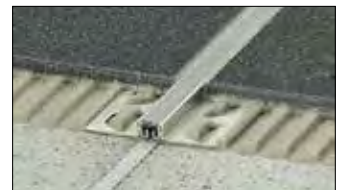
Schlüter®-DILEX-KS is a movement profile with edge protection consisting of lateral anchoring legs made of aluminium or stainless steel, which are connected to a replaceable movement zone made of soft rubber. (Product data sheet 4.8)
