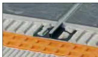
Schlüter®-DILEX-BWS is a movement joint profile with side sections of rigid, recycled plastic. The movement zone consists of soft CPE and creates the 5 mm wide visual surface. (Product data sheet 4.7)
