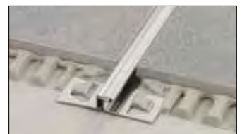
Schlüter®-DILEX-EDP is a stainless steel movement profile, which allows horizontal movement through a tongue and groove connection. (Product data sheet 4.16)
