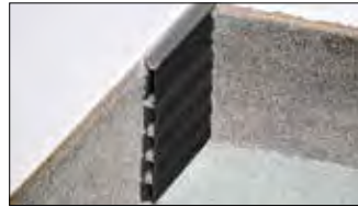
Schlüter®-DILEX-EZ 70 is a stress relieving and decorative profile with undercut side walls made of rigid PVC and a soft PVC expansion zone for use in screeds. The extension segments can be removed to adjust the profile height to the height of the assembly. (Product data sheet 4.2)
