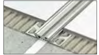
Schlüter®-DILEX-BT is a structural expansion joint made of aluminium with lateral joint connections to a sliding telescopic centre section. This allows for absorption of three-dimensional movement. (Product data sheet 4.20)
