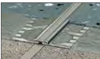
Schlüter®-DILEX-EKSB is a movement profile with edge protection for floor coatings and other thin floor coverings. It consists of lateral stainless steel anchoring legs that are connected to a fixed elastic insert of soft synthetic material. (Product data sheet 4.8)
