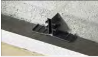
Schlüter®-DILEX-EP is a movement joint profile for application in floating or bonded screeds. The side sections consist of rigid, recycled plastic connected on the top and bottom with soft, grey CPE movement zones. (Product data sheet 4.5)
