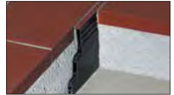
Schlüter®-DILEX-MP is an expansion profile with undercut sidewalls made of rigid, recycled PVC and a soft CPE expansion zone, complete with extension profiles for use in the laying of screeds. (Product data sheet 4.3)
