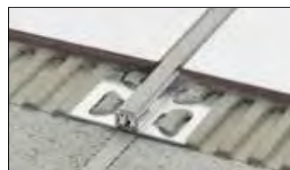
Schlüter®-DILEX-AKWS is a movement profile with aluminium side anchoring legs connected to a soft PVC movement zone. (Product data sheet 4.18)
