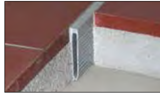
Schlüter®-DILEX-MOP is an expansion joint profile with serrated sidewalls made of rigid, recycled PVC and a grey, soft PVC expansion zone for use in screed applications. (Product data sheet 4.4)
