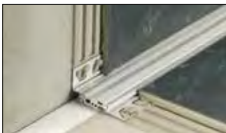
Schlüter®-DILEX-BTO is a structural movement and control joint profile made of aluminium for floor to wall transitions. The lateral joint connection of the sliding middle section of the profile is able to absorb three dimensional movement. (Product data sheet 4.20)
