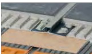
Schlüter®-DILEX-BWB is a movement joint profile with side sections of rigid, recycled plastic. The top movement zone is made of soft CPE and creates the 10 mm wide visual surface. (Product data sheet 4.6)
